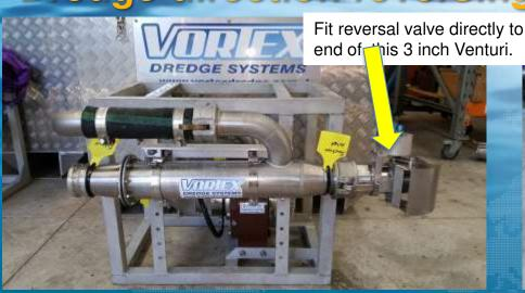
Or fit reversal valve to end of exhaust hose. Which ever suits your installation.
