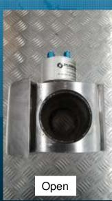
The venturi can be removed from the frame and installed individually on the ROV as shown below.
